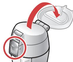
In the state the button unlocked, the cap lid opens by pressing the button.
